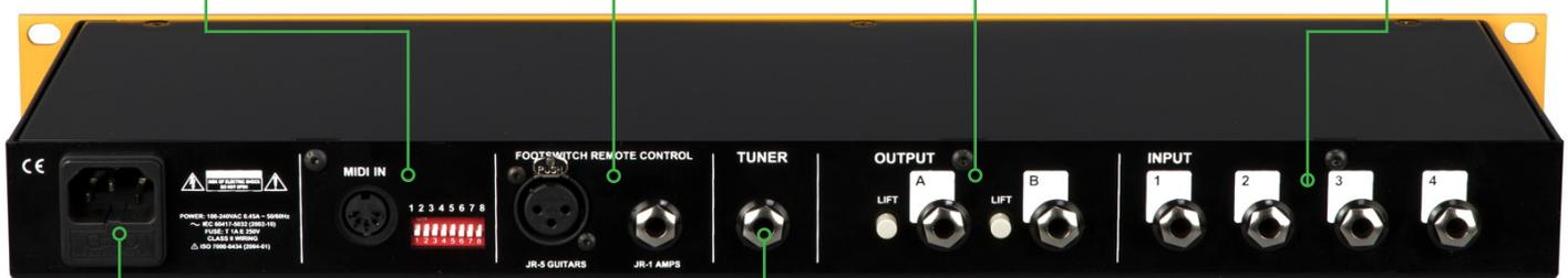
**IEC POWER:** Connection for standard IEC power cable. 120V/240V operation for international use.
