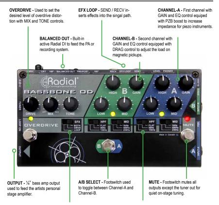
**EFX FOOTSWITCH ASSIGN -** Sets the footswitch function to activate the overdrive, effects loop or both.
