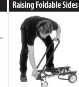
Firmly press down on release cable while raising other end of foldable side as shown.
