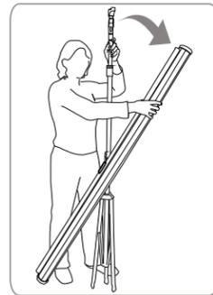
Lift the screen using the ring and place onto the top hook.
