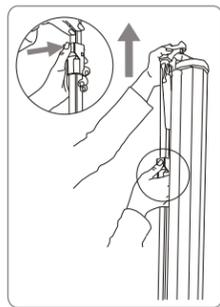
Raise the top hook using the coloured button to release the top locating pin.
