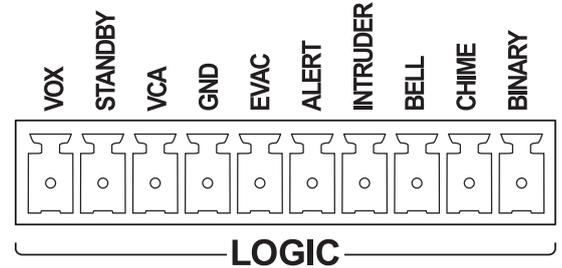
The table below shows the trigger combinations. Connect the appropriate logic input to the GND pin to activate the function.
