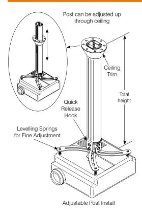
08 85 59 70 95 Ceiling Plate Mounting Hole Spacing
