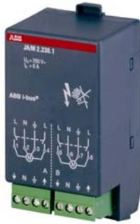
The 2-fold Shutter Actuator Module is a device for insertion in the Room Controller Basis Device. Using relay contacts, it switches two independent electric drives such as shutter motors or ventilation flap drives.
