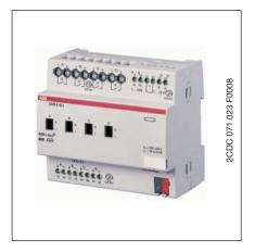
The ABB i-bus<sup>®</sup> Light Controllers, LR/S x.16.1 (x = 2 or 4) are KNX modular installation devices in ProM Design for installation in the distribution board on 35 mm mounting rails. The connection to the ABB i-bus<sup>®</sup> is implemented via a bus connection terminal on the device shoulders.
