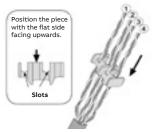
2.3 Ensure the end piece is located as close as possible to the edge of the jacket.
