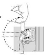
5 Disassembling the module from the supporting piece
