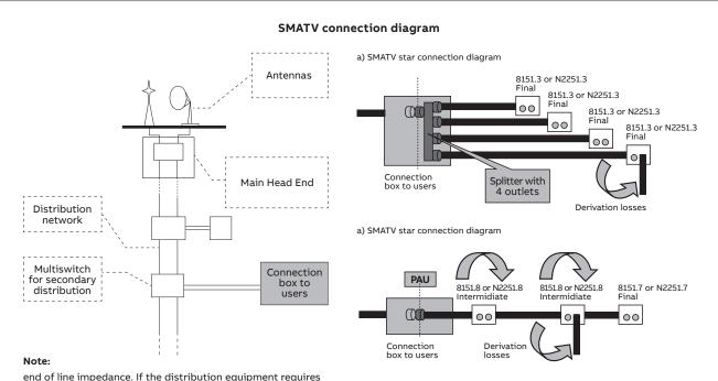
end of line impedance. If the distribution equipment requires outlets with end of line resistors, 8151.7/N2251.7 outlets must be used or add to 8151.3/N2251.3 outlets a termination resistor to close the line.
