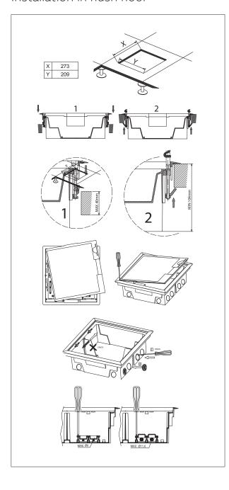
Installation of frame bracket T1393.4
