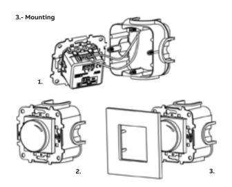
Turn the device in the correct installation position. The marks on the back side of the device, orients the correct top position.
