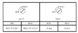
Figure 6: Exploded view of the selection potentiometers for the selection of light and time thresholds
