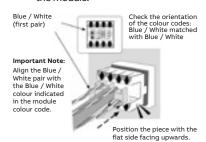
2.6 Unbraid the pairs, position and insert the cable in the module slots. Place the solid colour cable in the first slot of the pair.
