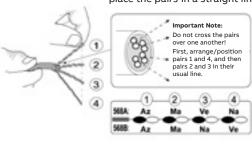
2.2 Position each of the four pairs in the holes of the end piece.
