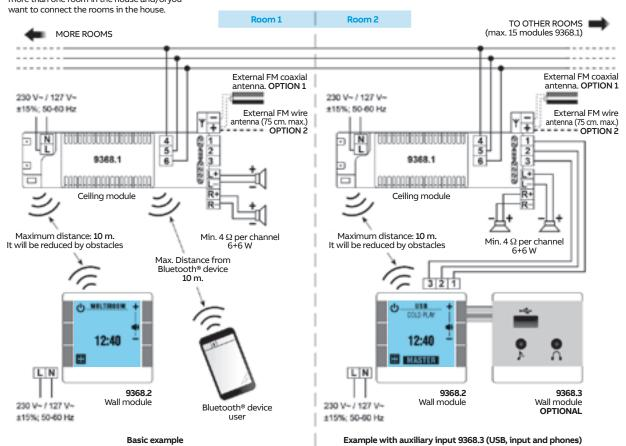
**NOTE**: Because these devices are radio frequency and to avoid interference, you should not install modules of the same reference or any other RF equipment that could interfere less than 1 m. away.
