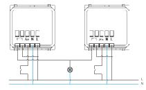
Figure 5: Parallel wiring diagram
