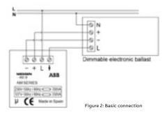
The maximum charge to be connected to the control terminals +/-should not exceed 50 mA.
