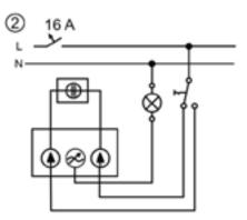
Operation in a two-way circuit
