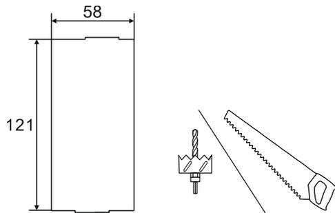
Fig. 9: Dimensions for mounting in hollow wall
