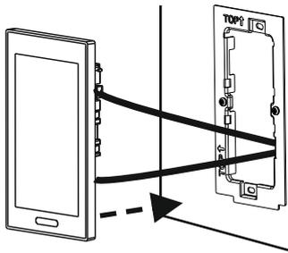
Fig. 21: Insert the ABB RoomTouch® 5, FM
