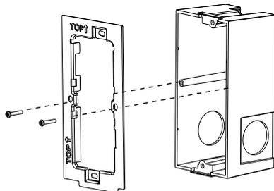
Fig. 10: Installing the frame
