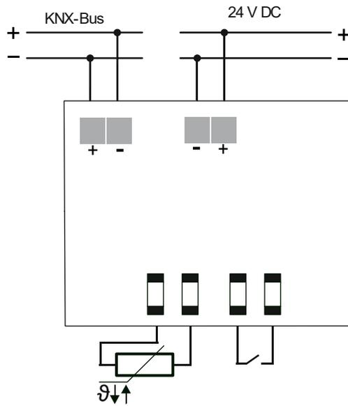
Fig. 5: Connection ABB RoomTouch® 5, FM
