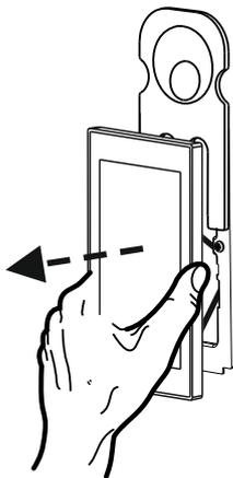
Fig. 24: Removing the ABB RoomTouch® 5, FM
