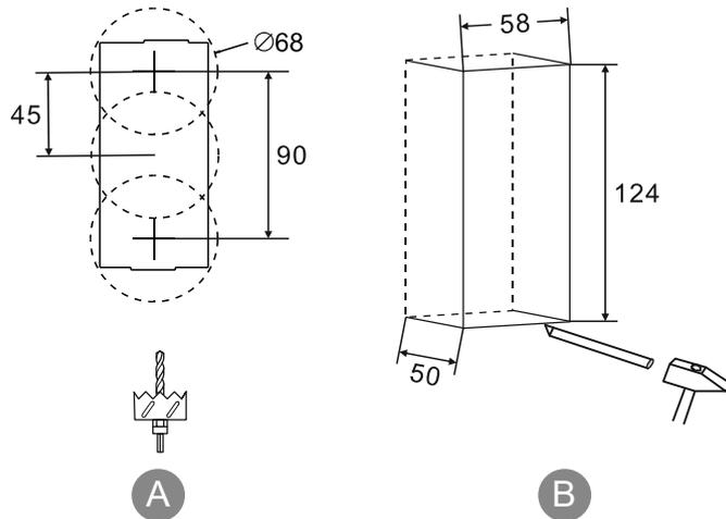
Fig. 15: Dimensions for mounting in solid wall
