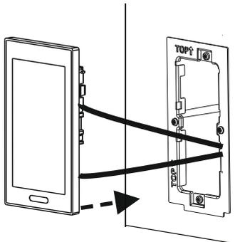
Abb. 14: Inserting the ABB RoomTouch® 5, FM
