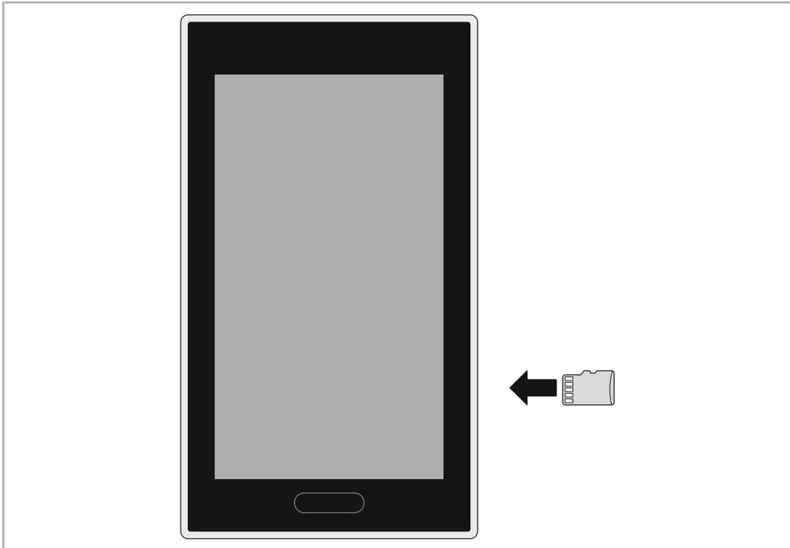
Fig. 38: Inserting the micro SD card (SDHC)
