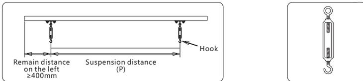
Hook the hooks to the middle circular holes on the left, middle and right hanging plates respectively, adjust the length of the hooks to the level of the screen, and complete the lifting; ( Note: The left and right hanging plates are the main stress points, and the middle hanging plate is the secondary stress point, and the middle hanging plate is only suitable for shell length  $6 \geq$  meters, less than 6 meters, no need to install the middle hook)
