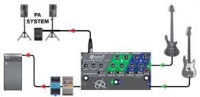
To take things one step further, the Bassbone OD is equipped with an effects loop. When pedals are connected in the loop you can use them with both instruments and choose to send the pre-effects signal (dry) or the post-effect signal (wet) to the PA.
