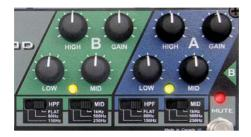
Each channel has two 3-position switches. The MID switch allows you to choose between three center frequencies. This is used along with the MID EQ control to shape your sound.
