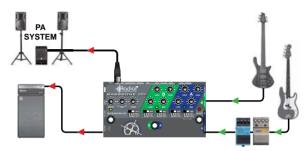
You could also introduce a series of pedals between the Bassbone OD's  $\chi^{"}$  output and your amp. This way the pedals can be used with both instruments and your amp but the effects will not be sent to the PA system.
