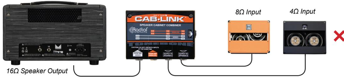
When connecting your cabinets in parallel configuration, the overall impedance decreases (two 8 $\Omega$  cabinets wired in parallel will present a 4 $\Omega$  load).
