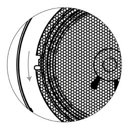
To reassemble, reinsert the grille following the reverse process and the front plate is simply pressed back into the speaker.
