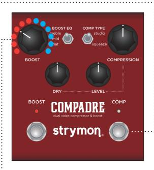
Turn the BOOST knob to select the function of the FAV/MIDI jack. The BOOST LED will change from RED to BLUE to indicate the current status as the knob is turned.
