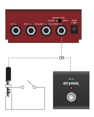
NOTE: Along with the knobs and toggle switches on the face of the pedal, the setting of the rear BOOST TYPE switch and the bypass state of BOOST and COMP are stored with the FAV setting.
