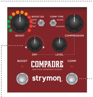
2 Sweep the **DRY** knob from 0-100% and back two (2) times. The **BOOST** LED will change colors at the extremes of the knob range and blink **RED** to indicate when the reset is taking place.
