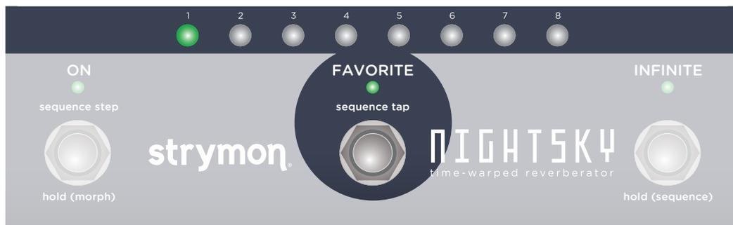
There are 16 onboard presets that are accessible by using the 8 **PRESET BUTTONS** on NightSky. They are arranged in 2 banks of 8 presets with different **PRESET BUTTON** colors indicating the selected bank.
