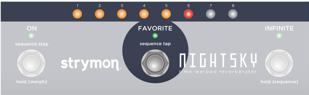
**NOTE:** A minimum of two active steps are required for the sequence to run.
