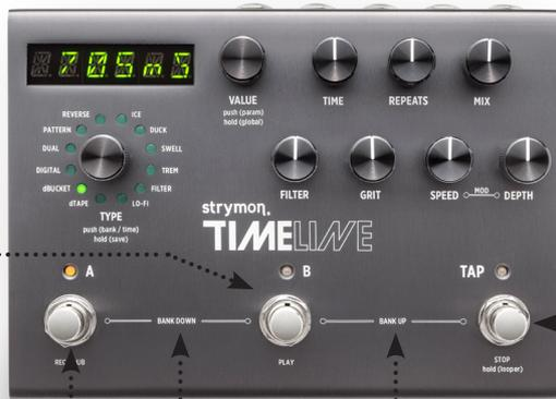
..... **FOOTSWITCH A:** Press to engage or bypass preset A of the current bank. Hold to activate infinite repeats.
