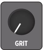
**BUCKET LOSS:** In dBucket, the GRIT knob takes the function of BUCKET LOSS. This controls the amount of bucket brigade “chip” loss at each stage in the dBucket algorithm, from no loss at minimum, to full noisy loss at maximum. Set to 3:00 to get maximum distortion loss with just a hint of noise. Increasing from 3:00 adds more noisy loss.
