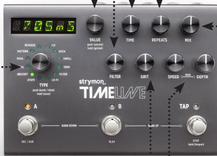
**MIX:** Adjusts the mix of analog dry signal to wet delay signal. The Mix occurs in analog. Set around 3 o'clock for a 50/50 mix.
