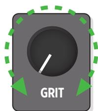
**GRIT:** The intensity of the Grit control will depend on the strength of the input signal. Hotter inputs will intensify the effect of the Grit knob in all modes. The volume of the wet signal may change as you increase the Grit control (getting louder or softer depending on the input signal strength). Use the MIX knob to compensate accordingly.
