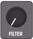
**FILTER:** In dBucket, the filter control makes the repeats either darker or brighter depending on preference. 12:00 is a neutral filter setting. Turning the filter clockwise makes the repeats darker and they will get progressively darker with each repeat. Increasing the bucket loss will darken the repeats even further. Turning the filter counterclockwise makes the repeats brighter by applying a ‘post’ high shelf EQ to the wet signal.
