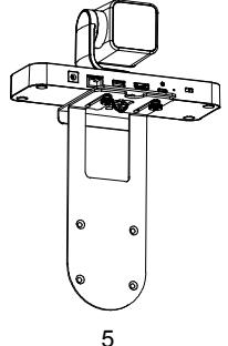
2. Using the thumb screw to fix the mounting brackets to the camera, as shown in figure below.
