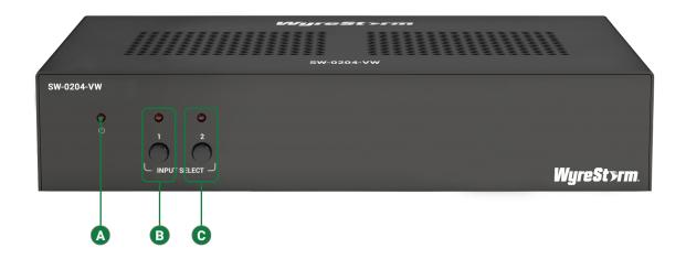
A Power LED Solid: The unit is powered On Off: The unit is powered Off
