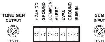
**24V DC / GROUND** This input pair is for connection to a 24VDC emergency power supply and is not switched by the front panel power switch.
