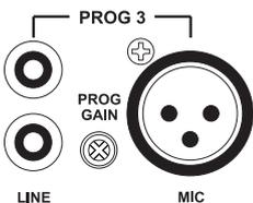
**LINE** The pair of RCA sockets accepts unbalanced line level inputs. Stereo signals are internally summed to mono.
