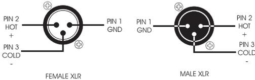
When wiring the outputs on the DigiPage as unbalanced, Pin2 should be used as hot and Pin1 as ground. Pin3 should be left open and NOT shorted to Pin1.
