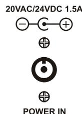
This 2.1mm x 5.5mm power socket accepts 20VAC or 24VDC. For DC, tip is positive.
