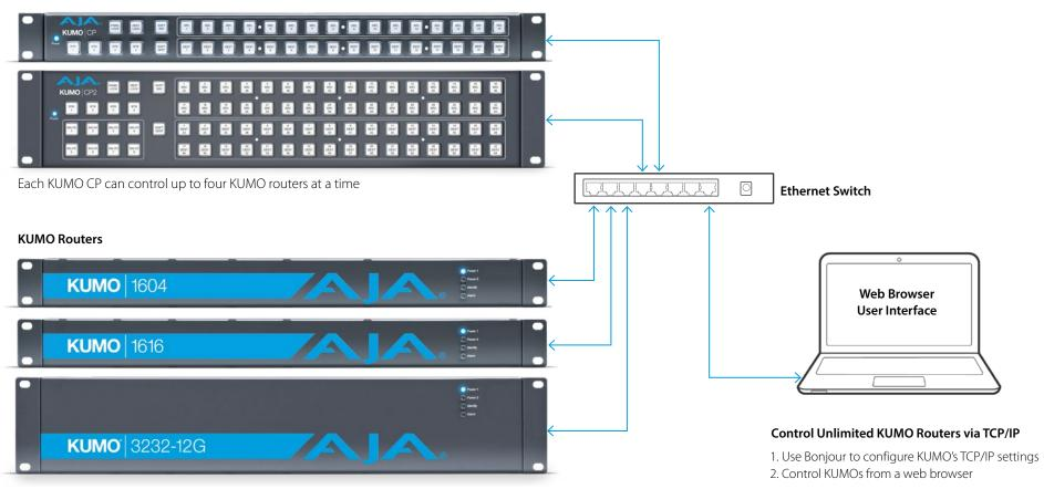
Each KUMO router can be controlled by multiple CP panels
