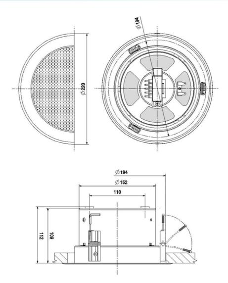
Measurements according to DIN IEC 268-5
