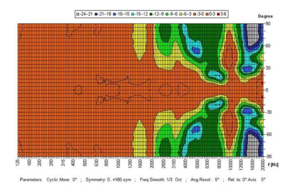
POLAR DIAGRAM — WITH SPAC-FD-E-50 FIRE DOME
