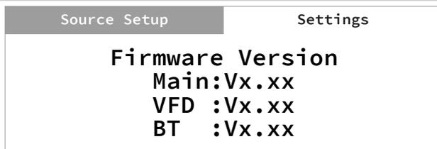
Firmware version details of Main (MCU), VFD (display) and BT (Bluetooth) are displayed. "x.xx" above stands for the version number of the particular firmware item.
