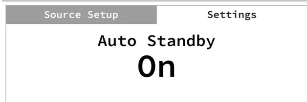
Auto Standby feature is an integral feature of C 388 that conforms to European ecodesign regulations. The C 388 can be setup to automatically go to standby mode if there is no user interface interaction and no active source input within 20 minutes.
