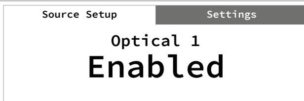
One can enable/disable a Source via this option. This is particularly useful if only few Sources are used and one directly selects the Source from the front panel, bypassing unused sources.
