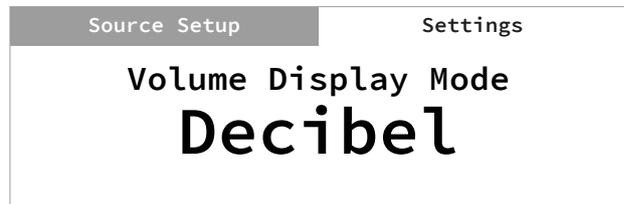
Volume Display Mode gives the user two options on how to display Volume level. Use < or > to select between "Decibel" and "Percent" Volume level display mode.
