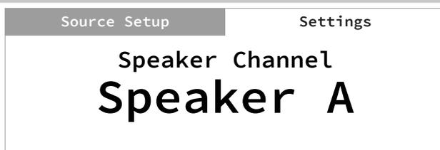
SPEAKER CHANNEL enables you to engage or disengage the speakers connected respectively to the SPEAKERS A and SPEAKERS B terminals on the rear panel.
