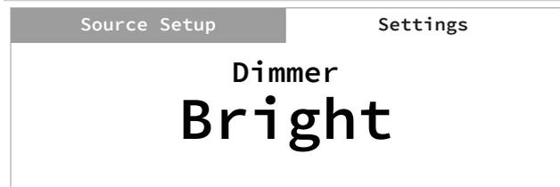
DIMMER function makes it possible to adjust the brightness level of the front panel display.
