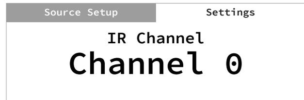
The C 388 has the capability to operate via Alternate IR channel. This is useful if you have two NAD products that can be operated by similar remote control commands. With alternate IR Channel, two different NAD products can be controlled independently in the same zone by setting each one to a different IR channel.
