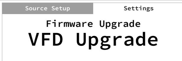
Select Firmware Upgrade to initiate VFD Upgrade or BT Upgrade. At each upgrade mode, select "Yes" to start upgrade process or "No" to retain current firmware.
