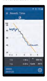
The standard reverberation time measurement determines T20 or T30 in octave bands from 63 Hz - 8 kHz. The values of a measured position or of an entire room are averaged on the XL3. The optional Room Acoustics Package extends the Acoustic Analyzer to 1/3 octave band resolution, T15 or EDT. Use either an impulse source or an interrupted pink noise as the test signal.
