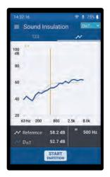
The optional Building Acoustics module enables direct determination of airborne and impact sound insulation, according to ISO 16283, while you are on site. Measure in the source and receiving rooms and see the sound insulation results on the display. A detailed measurement report is easy to create with the optional Sound Insulation Reporter PC Software.
