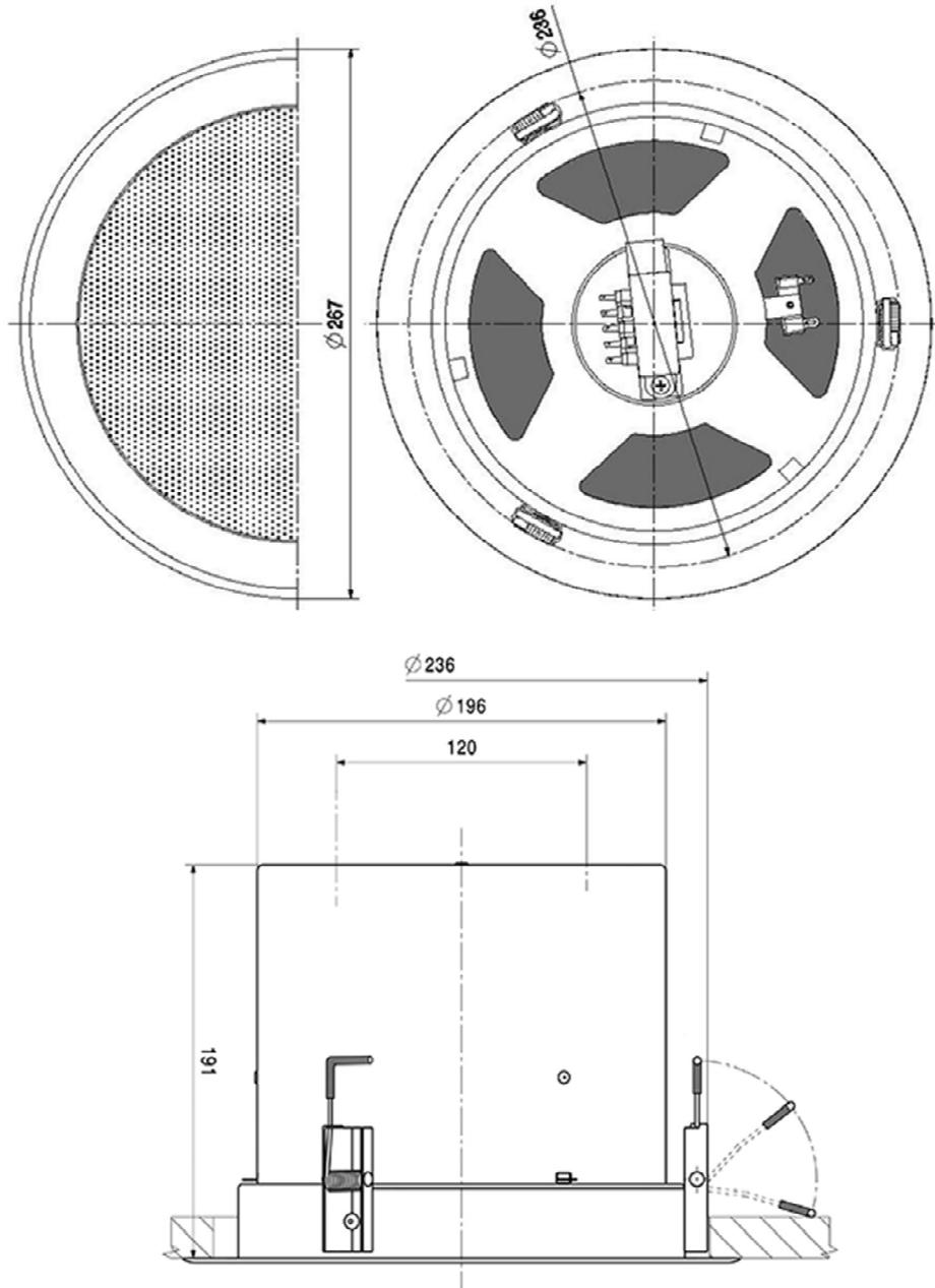
Measurements according to DIN IEC 268-5
