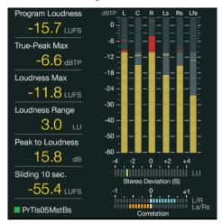
Regardless of the Main Section view on the left side, the screen will show various levels and metering feedback on the right-hand side of the screen. This information can be edited on a preset basis using the 6th button (Edit). See the 'Editing Presets' section for more details.
