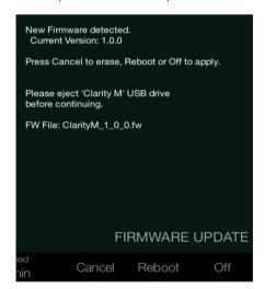
Eject the Clarity M from your computer first, then either press cancel to abort the update, or press reboot or off to apply. When you turn the unit on again it will be running the new firmware.
