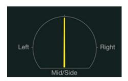
A center-balanced mono signal with no width will appear as a single line.
