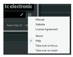
Take over on focus - When this is selected, a newly-created instance of the plug-in within a DAW project will automatically be connected to the hardware unit. Otherwise, an instance of the plug-in that was already active will take priority and remain connected.
