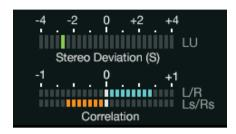
This section has 2 horizontal bar graphs that appear in the lower right corner of the screen. The upper graph shows the downmix deviation meter, and the lower shows correlation.
