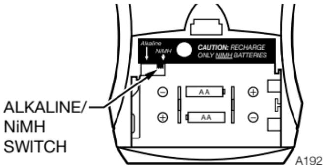
3. Insert 2 AA batteries over the fabric strip. Note correct polarity (+/-).
