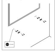
Adjust the two thumbscrews and hang Collabo carefully onto the wall. Make sure it will slide down into both brackets properly.
