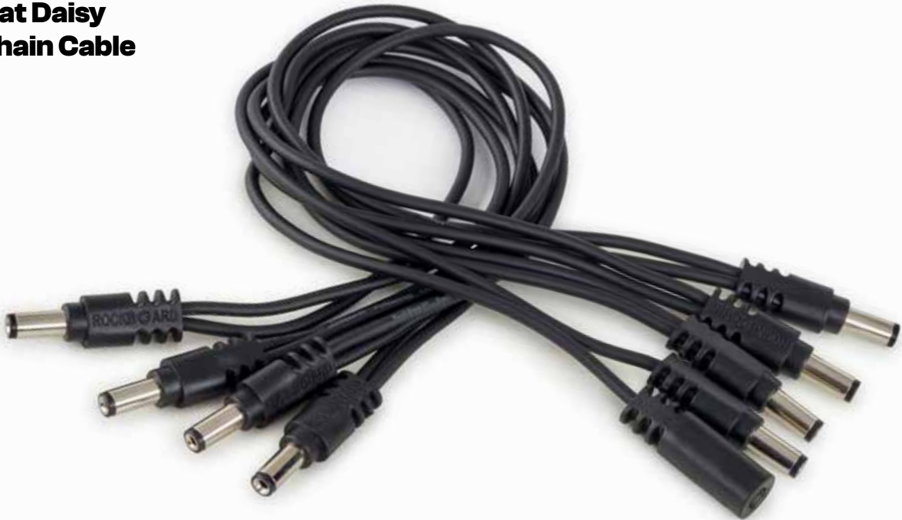
3 Flat Daisy Chain Cable Designed like instrument cables with twisted copper shielding to minimize electrical interference. 5.5 x 2.1 mm barrel plugs. Length between plugs: 30 cm / 11.81". Plug dimensions (L x W x H): 20 x 9 x 10.5 mm / 0.78" x 0.35" x 0.39" (angled) 20.5 x 11 x 8.5 mm / 0.79" x 0.43" x 0.31" (straight).
